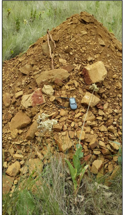
Plate 1: Typical soil profile encountered throughout the site (RW09) with clayey sand colluvium overlying clayey silt residual shale. (13 March 2014).
