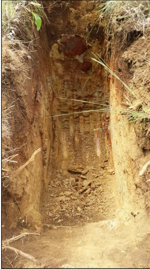
Plate 1: Typical soil profile encountered throughout the site (RW09) with clayey sand colluvium overlying clayey silt residual shale. (13 March 2014).
