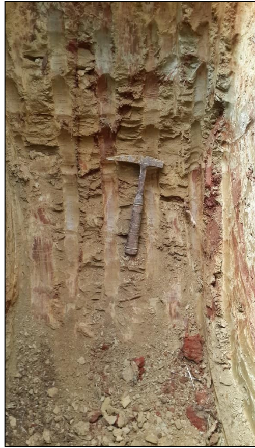
Plate 2: Shallow refusal of TLB on completely weathered very soft rock shale. (13 March 2014).
